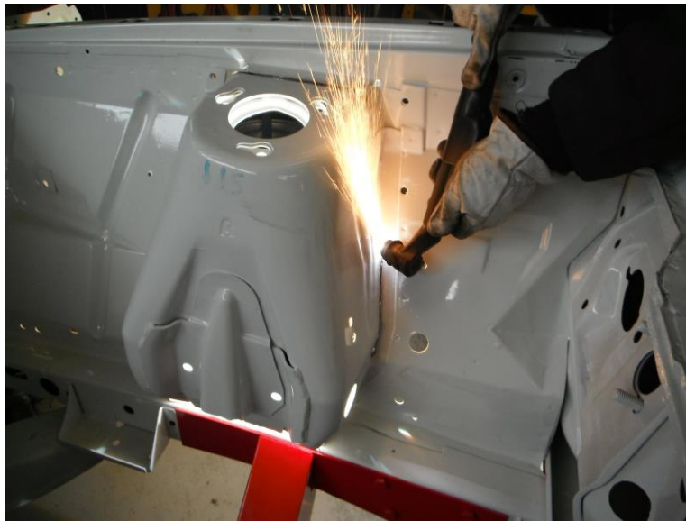
C. Vertical cut is made between radius on tower and skirt panels at rear of the tower.
