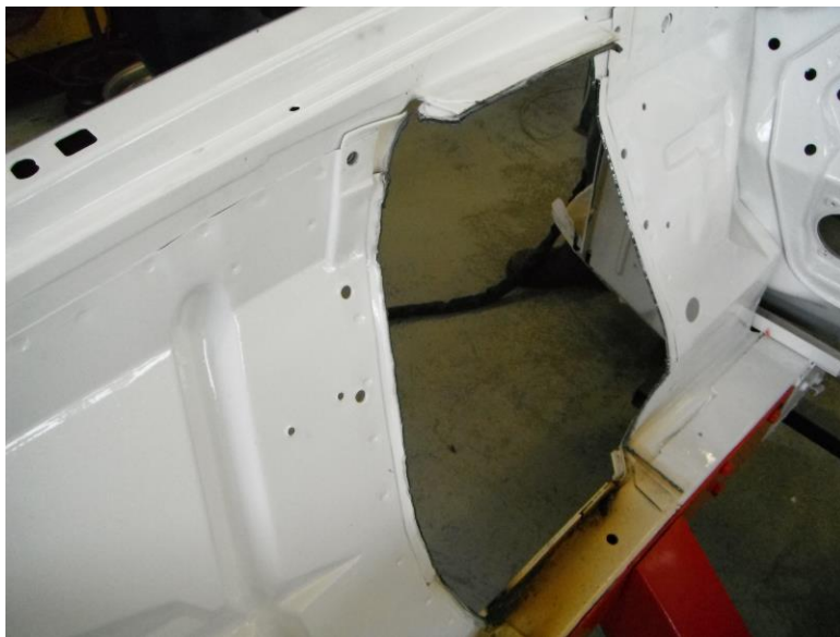
D. This shows the cut away of the lower edges of the tower from the frame rail, Now grind all edges smooth to allow fitment of shock tower filler panel, Inc top of rail.
